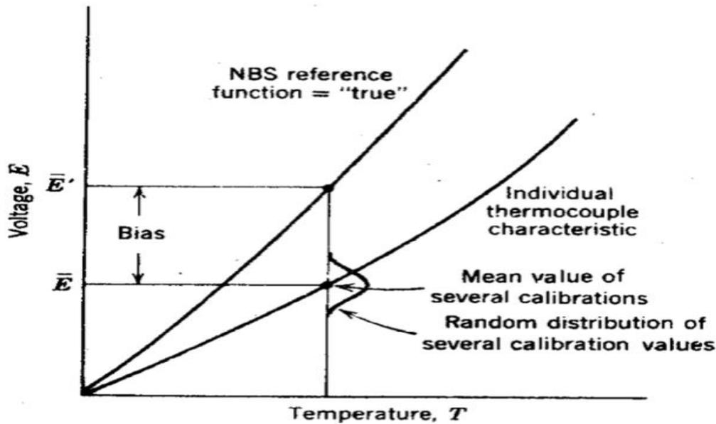
**Figure 2.1 Systematic and random errors illustrated for case of thermocouple calibration [2]**
