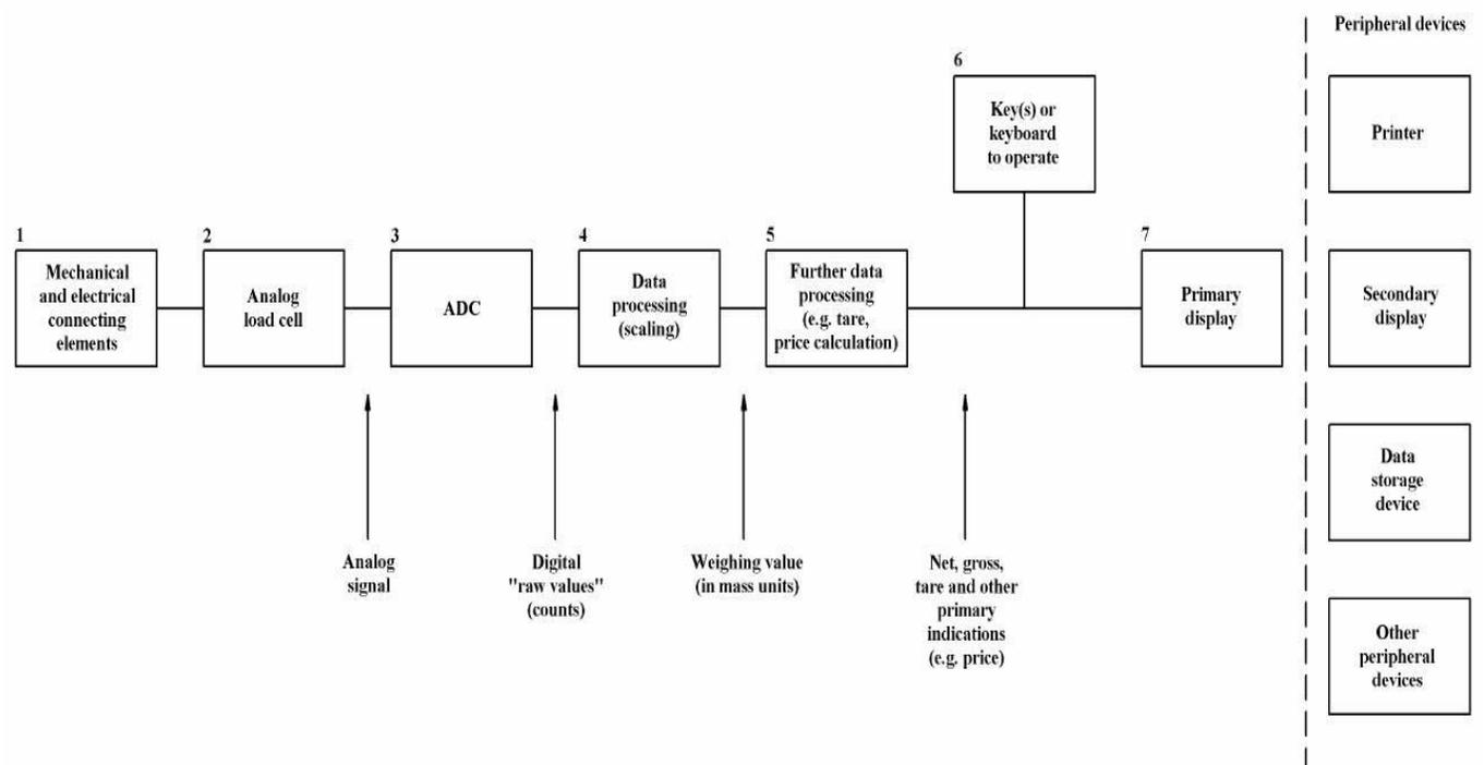
**Figure 1:** Definition of typical modules according to 1.2 [2].
