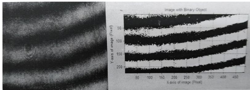
Figure (7) fringes pattern by ESPI technique and related binary interference fringes pattern.
